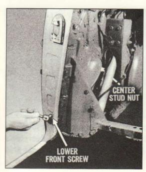
To adjust window guide channel in case of bind at lower end — loosen guide lower front screw and center stud nut. Adjust stud to move channel IN OR OUT as required. Tighten stud nut and screw.
