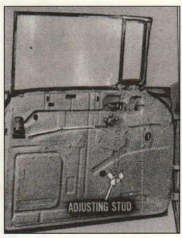
To adjust front of window upper frame IN OR OUT for contact with roof rail weatherstrip and to adjust lower portion of window division channel FORE OR AFT — loosen channel lower adjusting stud nut and adjust stud as required. Tighten nut.
