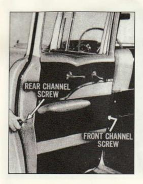
To adjust for freedom of glass movement in run channels — loosen front channel screw or rear channel screw at lower ends and move IN OR OUT as required. Tighten screws.
