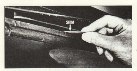
To move side rail weatherstrip down for better contact with top of glass frame – loosen weatherstrip nuts and install weatherproof tapered shim or shims at required area. Tighten nuts.
