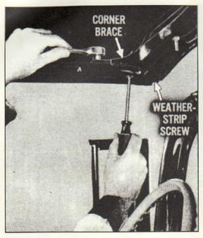
If the front roof rail is too far FORWARD OR REARWARD to properly engage the windshield header, raise top slightly. Remove weatherstrip end screw and loosen corner brace attaching screw and bolt. Then...
