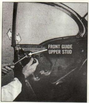
For IN OR OUT adjustment at front of window — loosen the front guide upper adjusting stud nut and adjust stud as required. Tighten nut.
