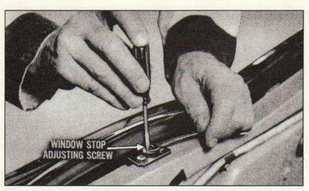
To limit the "up" travel of the window - adjust the window stop adjusting screw as required.
