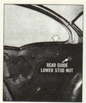
For IN OR OUT adjustment at rear of window — loosen the rear guide channel lower adjusting stud nut and adjust stud as required. Tighten nut.
